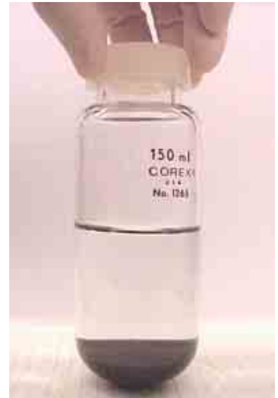
Alum-flocculation to remove colloids (Ghosh et al., ES&T 2000)
